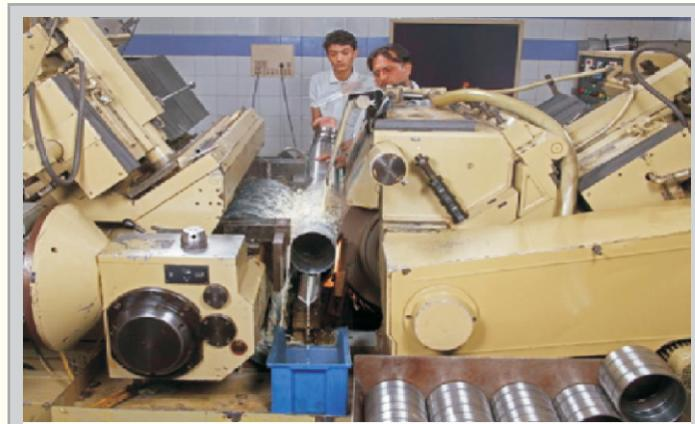
The OD grinding process is carried out using imported machine of reputed make, Microsa- Germany. The OD is the reference diameter for the next stage of track grinding, where the grinding is done with shoe centerless system. So the OD accuracy helps in building a good accuracy on track also.
