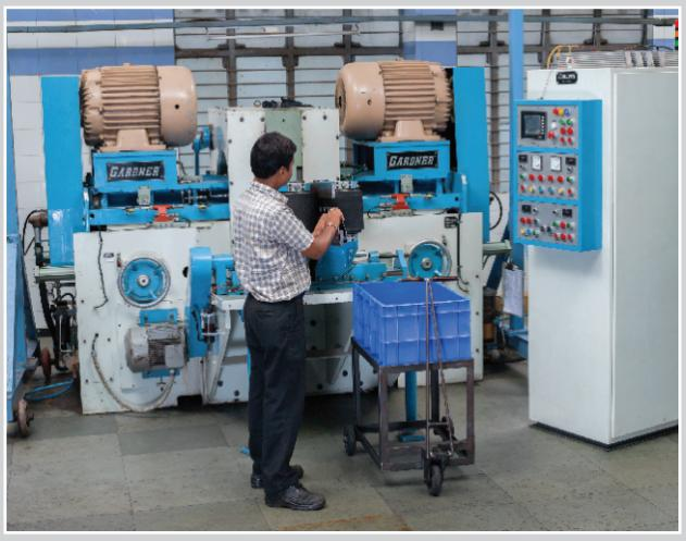
The face grinding is the first process in the PFC of bearing parts. The ground face generated after this process is the reference for all subsequent grinding processes & stands as a reference for achieving the accuracies at every stage. We control a close accuracy of Face flatness & parallelism between two side faces, using the world renowned machine for this process, Gardner USA. This machine is fitted with through feed system with high productivity and very high accuracy
