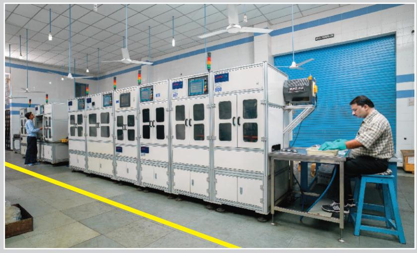
Our fully automatic assembly line includes demagnetising, washing, inspection for dimensional as well as visual parameters (roller missing), Vibration Testing, Laser Marking, drying and oiling. All these operations are fully automatic and inter-connected. The dimensional inspection is carried out by PULCOM (Japan make) gauges. Our assembly operations are carried out in a complete enclosure and dust-free environment.
