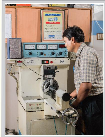
We have imported noise level testing machines, which are used for checking the noise & vibration of ball and roller bearings. These equipments have low band, medium band and high band vibration measuring facility, which enables to identify the control of quality parameters of various bearing components. They help in upgrading the bearing performance.
