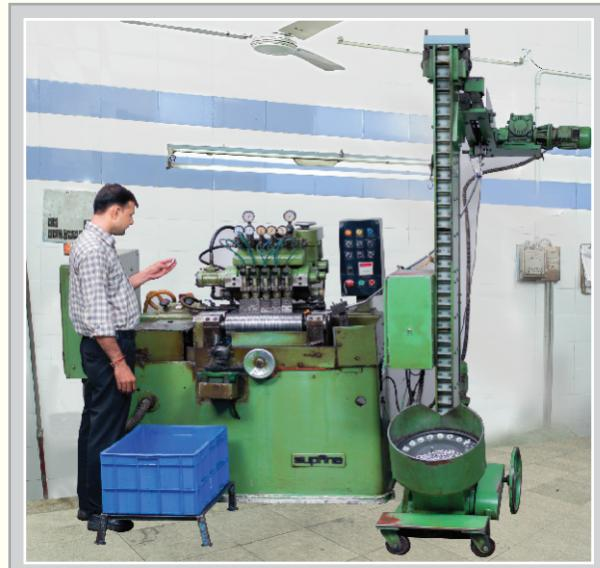
TURBO has world renowned super finishing machines of Supfina-Germany make for super finishing of rollers, which gives improved surface finish on roller, along with cambered profile - a unique feature with supfina machines.
