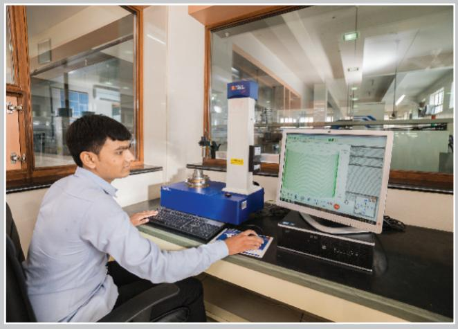
Talyrond - Taylor Hobson Ltd. (U.K.) make: This world renowned quality appraisal equipment is used for checking the roundness, squareness, concentricity, cylindricity, flatness and coaxiality of bearing components, which ensures running accuracy for longevity life of **TURBO** bearings.
