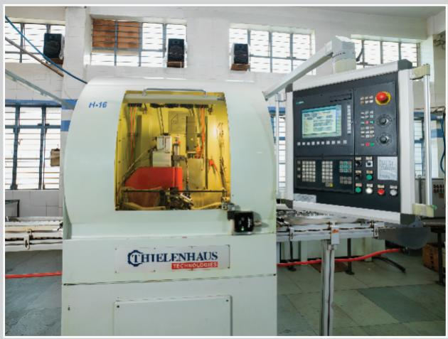
TURBO has excellent superfinishing machines of THIELENHAUS (German Technology), to achieve high degree of surface-finish accuracy of raceways and lip. These machines are equipped with special cycle to generate logarithmic profile.
