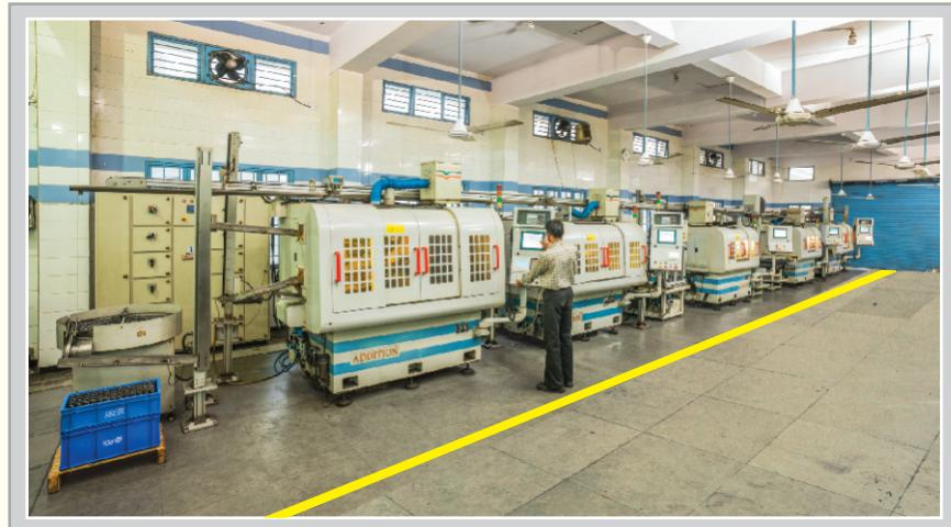
Turbo has installed fully automatic, inter-connected manufacturing lines with CNC grinding as well as CNC superfinishing machines, for Tapered Roller Bearings, Cylindrical Roller Bearings as well as for Ball bearings. The lines are equipped with In-process gauges as well as post process gauge for consistent quality. Size and geometrical tolerances are achieved with high accuracies.
