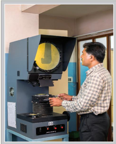
We have profile projector, which is used for checking/controlling the profiles of grooves, butting radius, etc., at turning stage.
