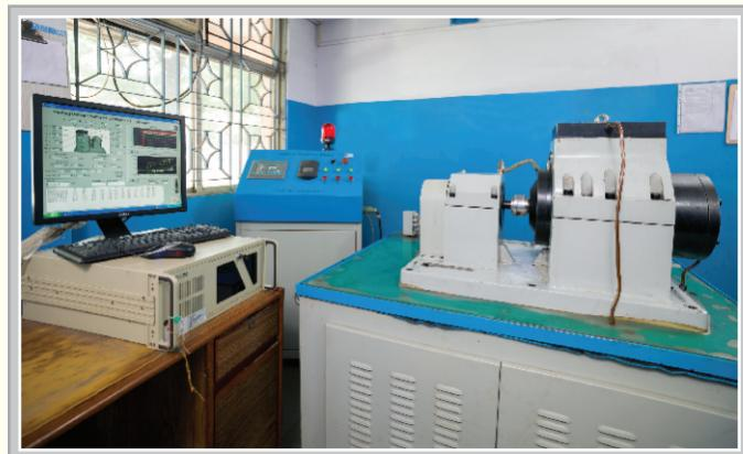
We have imported Bearing Endurance (Life) Testing Machines. These machines are suitable for testing Radial Bearings & Tapered Roller Bearings. These machines are equipped with programmable controls & monitoring systems to monitor vibration level, temperatures & speed of Bearings under test.
