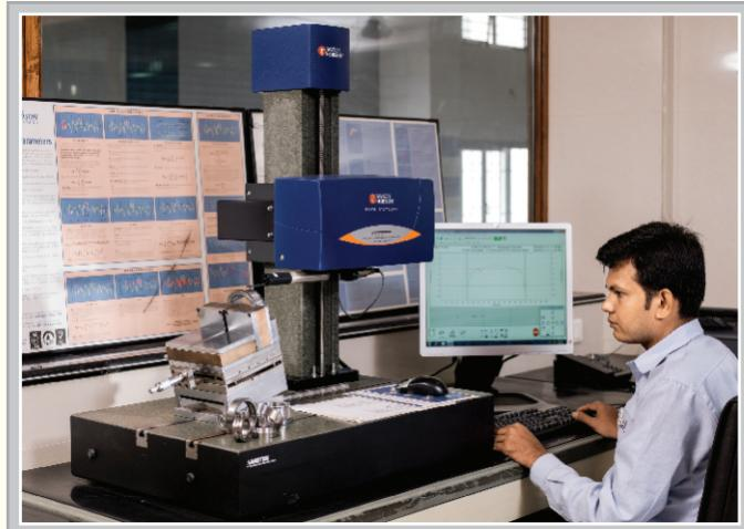
We have latest version of Form Talysurf (Form and Surface Finish Measuring machine) from world famous Taylor Hobson Ltd. (U.K.). This machine is used for checking Micro geometry. It evaluates parameters like Form geometry and surface finish of components. This control helps for improving the quality and product performance in the field. Our R& D continuously makes improvements in these accuracy parameters of races & rollers, to enhance field performance of **TURBO** bearings.
