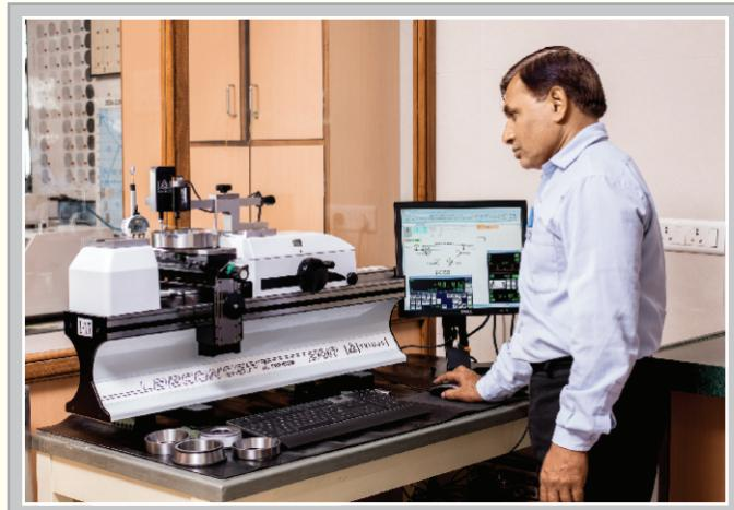
TURBO has installed a Universal measuring machine from TRIMOS - Switzerland. This machine gives absolute value of internal dimensions, external dimensions and angles of rings and rollers, measured as per international standards. This machine is used to calibrate the bearing components as per designed dimensions.
