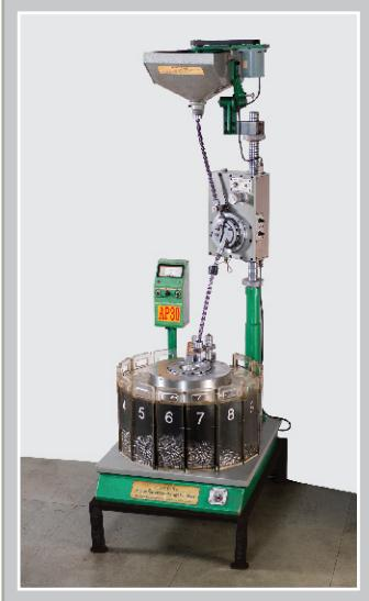
We have imported automatic roller grouping machines for Tapered rollers. These machines have facility to group the rollers within 1 micron grading. The close grading gives uniform load distribution in the bearings for longer life.
