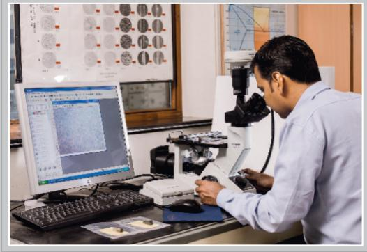
We have latest version of Metallurgical Microscope - Olympus (Japan make), with image analyzer software, used for checking the microstructure of bearing components. We maintain consistent quality of micro structure as per standard norms, in prime raw material as well as in heat treated rings, rollers & balls with reference to STAHL-ELSEN-PRUFBLATT 1520, (SEP-1520) German chart, for following:
