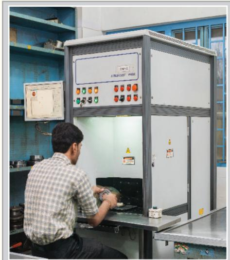
TURBO has Laser marking machines (IPG - German Make), which apart from marking the bearing number, also used for marking the Batch code (month and year code) on the bearings. This ensures the traceability of TURBO bearings up to field life.
